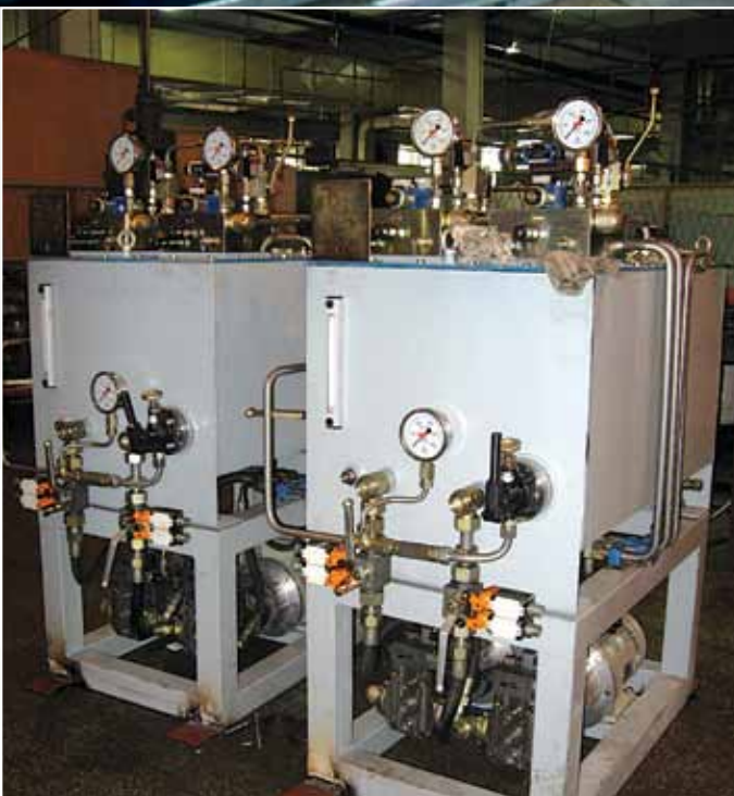
Hydraulic aggregate for sectoral gate drive
