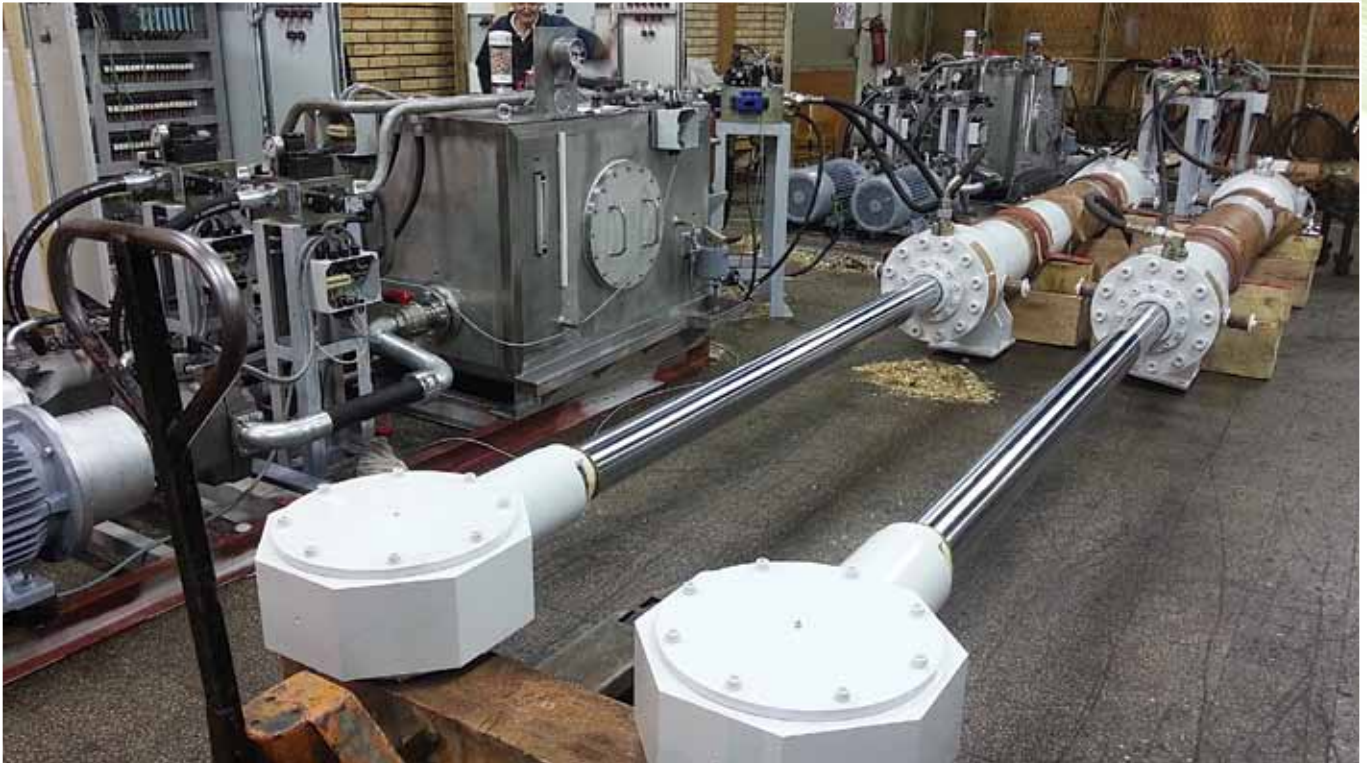
Electro-hydraulic system factory testing
