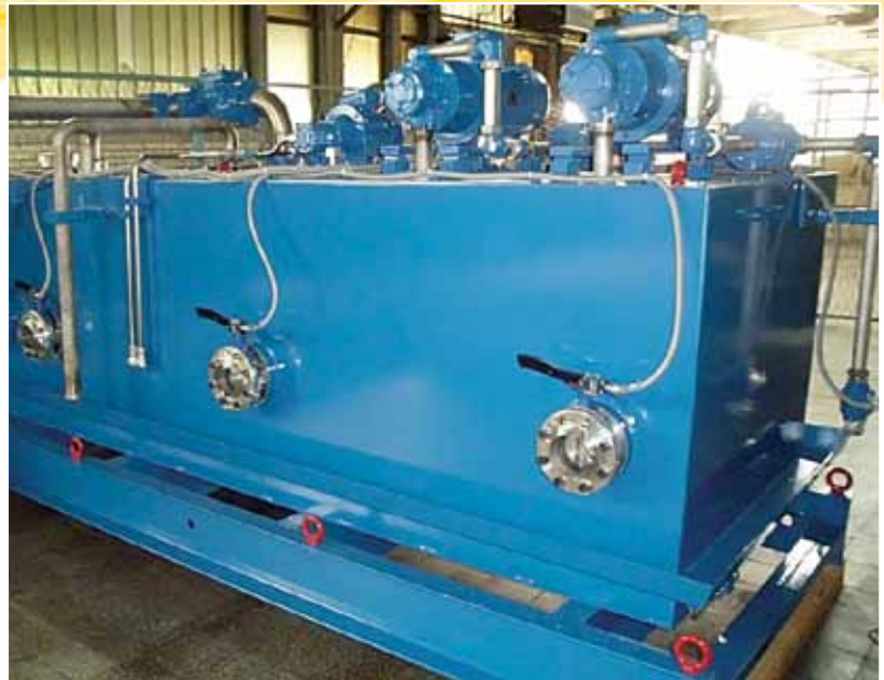
Hydraulic reservoir of furnace serving hydraulic system
